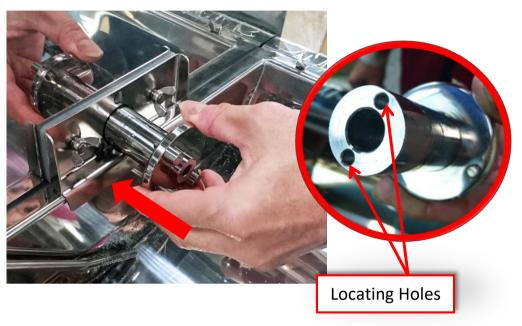
(Step 6) Reassemble the Rotating Plate Reassemble the ROTATING PLATE by aiming at the locating rod.
