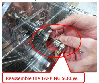
(Step 8) Reassemble the Injection Device Loosen up the TAPPING SCREWS circled on the photos and then lift up the INJECTION DEVICE to remove it.
