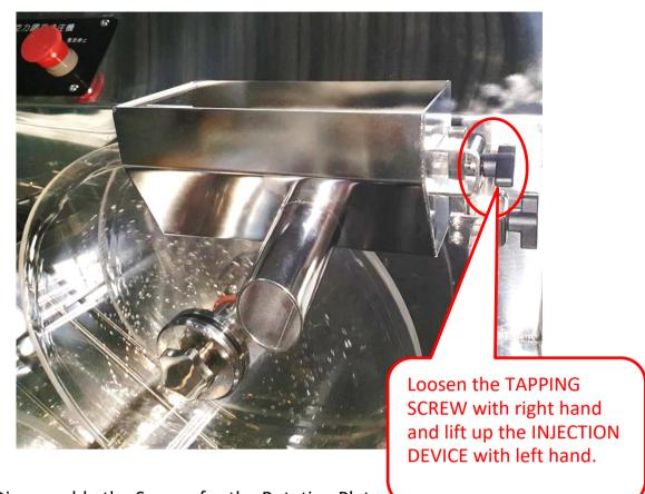
(Step 2) Disassemble the Screws for the Rotating Plate
