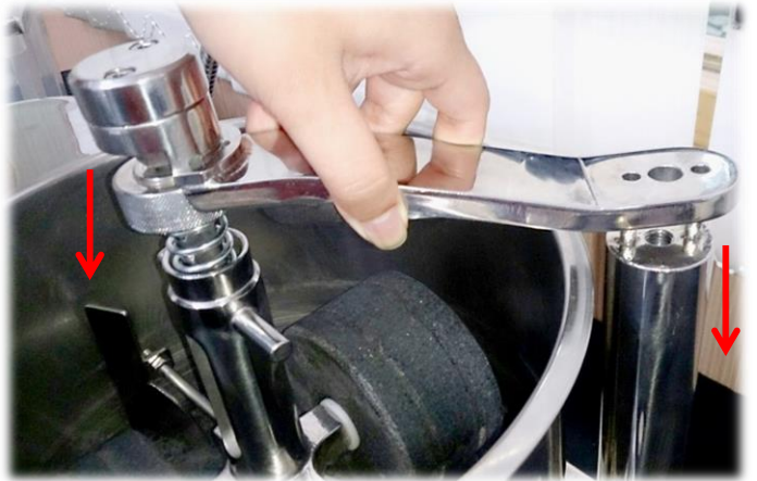
4. Install the positioning support. (Align one end with the positioning hole and align the other end with the two positioning rods. Put pressure on the positioning support and verify if the positioning support is well installed.)
