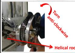
Push up the helical rod lock and hold it while turning the grinding disc anti-clockwise with the given wrench to remove it. Put down the wrench and remove the grinding disc with two hands to avoid dropping the grinding disc.
