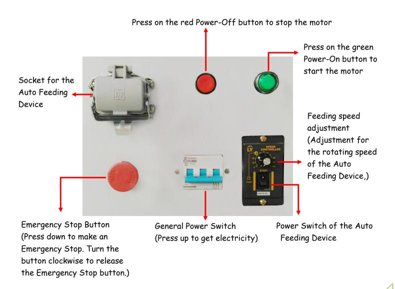
**%To prevent over-heating the motor, please <u>SWITCH OFF</u> the General Power Switch by pressing down the blue part.**
