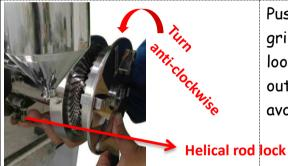
Push up the helical rod lock and hold it while turning the grinding disc anticlockwise with the given wrench. After loosen up the grinding disc, put down the wrench and turn out the grinding disc anticlockwise with two hands to avoid dropping it.
