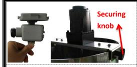
After switching off the power, remove the auto feeding device: Unplug the electrical cord located on the electricity control area. Loosen up the two securing knobs. Remove the auto feeding device.
